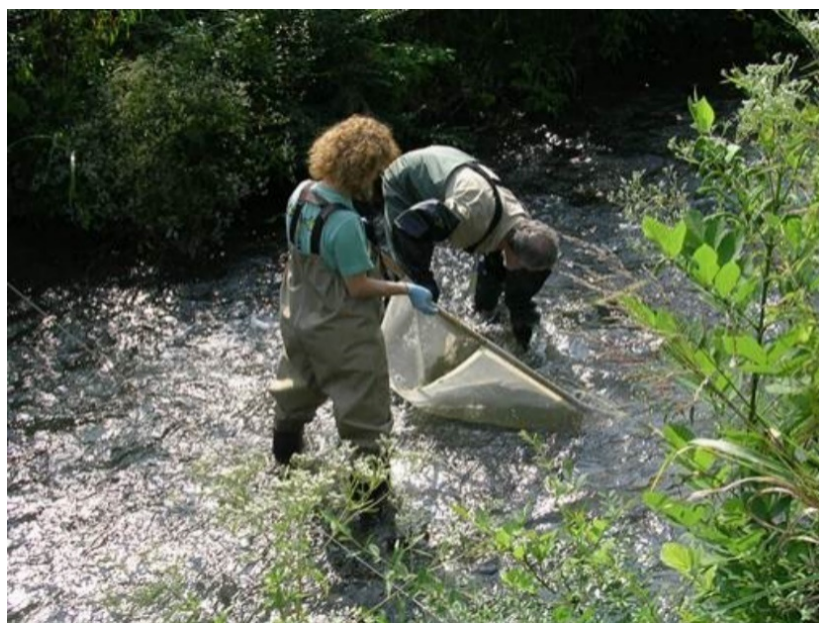
Figure 3.44. Sampling for benthic macroinvertebrates with TDEC protocols
